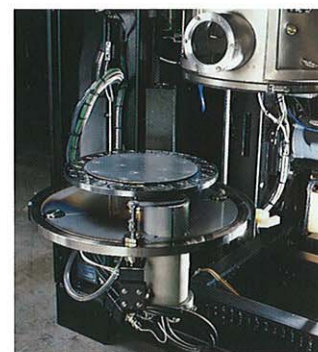
Substrate carrier swings out for loading
