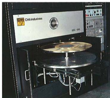
Substrate carrier rolls out for loading
