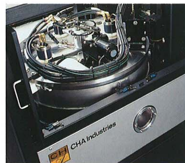
Upper cathode/fixture plate swings out for service
